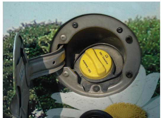
Figure 32. Bi-Fuel Vehicle Gasoline Fill Connection
