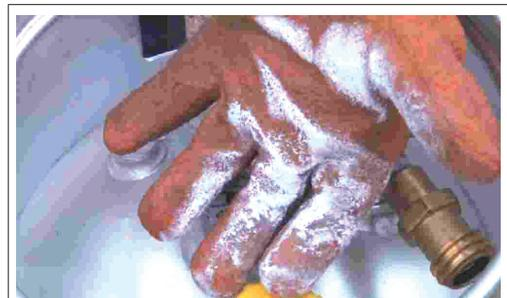
Figure 8. Frost on Vinyl Glove-Protected Hand
