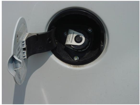
Figure 37. Filler Valve Dust Cover
