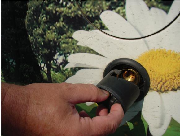
Figure 36. Filler Valve Dust Cover
