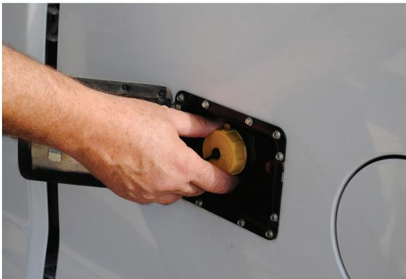
Figure 31. Bi-Fuel Vehicle Propane Fill Connection
