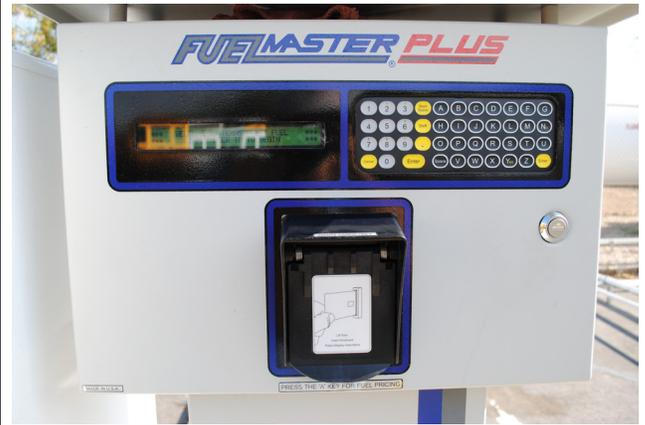
Figure 20. Customer Credit Card Interface and Display Panel
