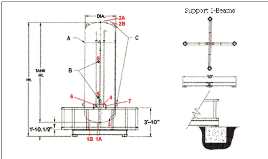
**Figure 14. Vertical Tank Specification Drawings and Foundation Partial Detail**
