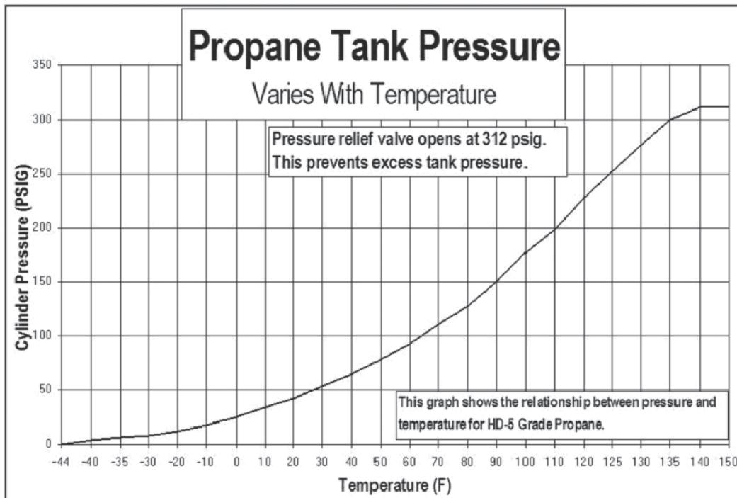
Figure 7. Vapor Pressure of HD-5 Propane
